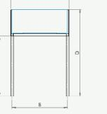
A tensile fabric wall mounted single pitch canopy with tubular steel frame
